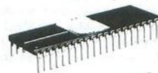
L SUFFIX CERAMIC PACKAGE CASE 715
